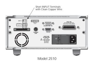
**NOTE** The characterized  $1\Omega$  resistor can be used in place of the shorted INPUT terminals, if desired. Enter the characterized value of the  $1\Omega$  resistor at the RES VALUE prompt.
