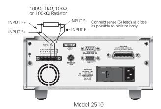
3. Select THERMISTOR, then press ENTER. The instrument will display the following: THERMISTOR CAL  $100\Omega$   $1k\Omega$   $10k\Omega$   $100k\Omega$
