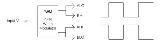
B. Pulse-Width Modulator Waveforms
