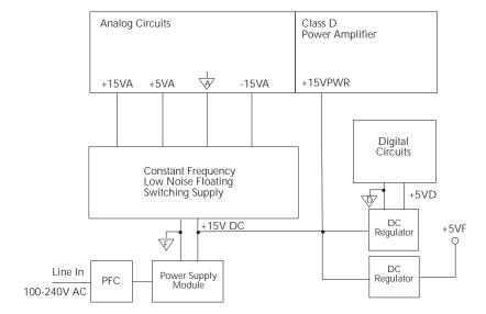
The integrated switching power supply module provides all power for the instrument while providing universal inputs and power factor correction for the 120/240V line. The +15VPWR voltage from the module powers the output stage directly, and this supply voltage is further regulated to develop a +5VF (floating) supply voltage and the +5VD (digital) voltage that powers the digital circuits.
