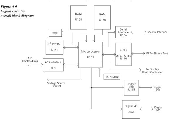
The core digital circuitry uses a Motorola 68332 microcontroller (U163) running at 16.78MHz. The memory configuration includes a flash EEPROM (U168) and a RAM (U160). Flash ROM support allows internal firmware upgrades using either the serial or GPIB port for downloading new firmware. All calibration constants and the saved setups are stored in a separate serial EEPROM (U141).
